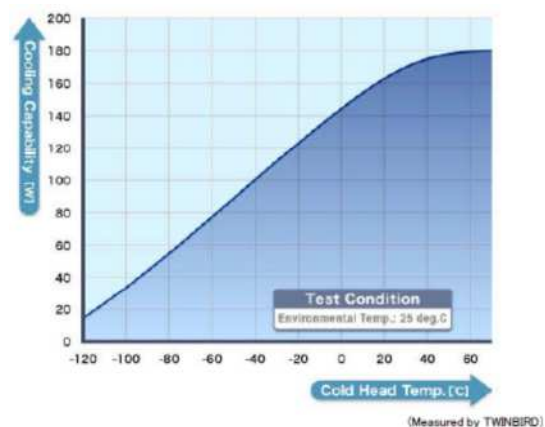
Figure 6.12 Refrigeration capacity variation as a function of temperature (Twinbird).
