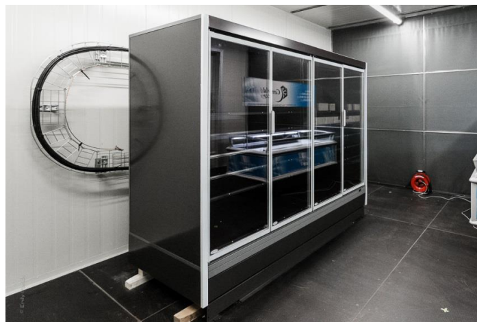
Figure 13-11: Climatic test room for refrigerated display case.
