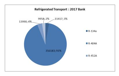
Figure 12-6: Sharing of refrigerant banks in refrigerated transport in 2017 (source Cemafroid) and in 2016 (source Inventories 2016, before R-542A introduction).
