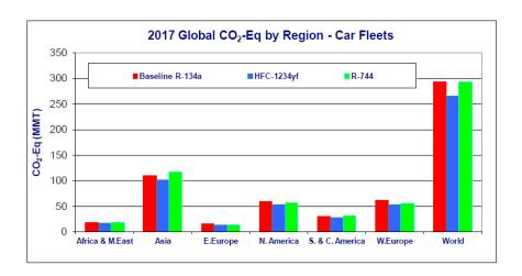
Figure 9-1: Evaluation of total equivalent CO<sub>2</sub> emissions (direct + indirect LCCP meaning) of fleets of mobile air conditioners assuming the implementation of alternatives to all new vehicles as of 2011 (Source: Papasavva, 2014).
