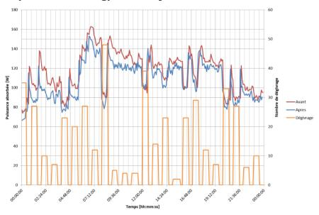
Figure 13-6: Evolution of the absorbed power compared to defrosting schedules of the medium and low-temperature refrigeration units.
