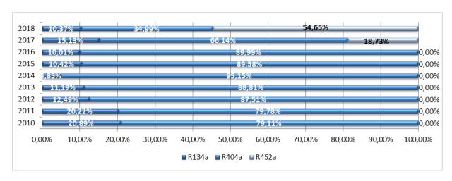
Figure 12-3: Synthesis of ATP attestations delivered for new vehicles per type of refrigerant.
