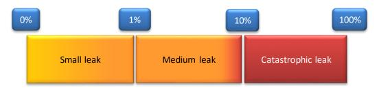
Figure 3-5: Leak typology as a function of leak diameter/piping diameter ratios.
