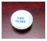
Figure 13-1: Temperature recorder.
