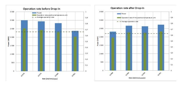
Figure 13-5: Daily energy consumption compared to the operation rate of the medium-temperature refrigeration unit before and after retrofit. In blue the daily energy consumption in kWh (left axis. In green the operation rate (right axis).
