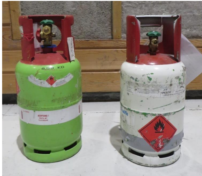
Figure 38: R-32 recovery cylinder (left) and R-32 fluid cylinder (right)
